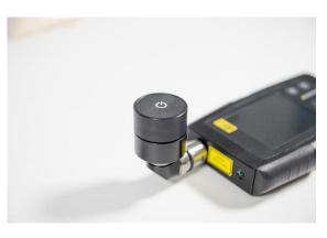
Place the top of the Active sample holder onto the mounted bottom part that is attached to the Serstech 100 Indicator hand-held Raman spectrometer.
