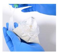
Collect sample particles using the swab stick. After this step, please very carefully remove the swab stick from the sample bag and place it back into the sample preparation bottle containing the solvent Methanol.
