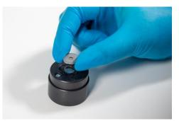
Now, place the washer on the center of the Active sample holder.
