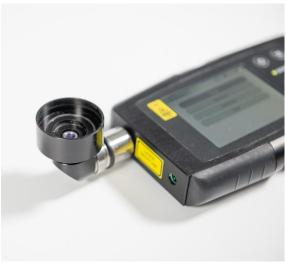
Mount the bottom adaptor of the Heroin ID device onto the Serstech 100 Indicator pointing up.
